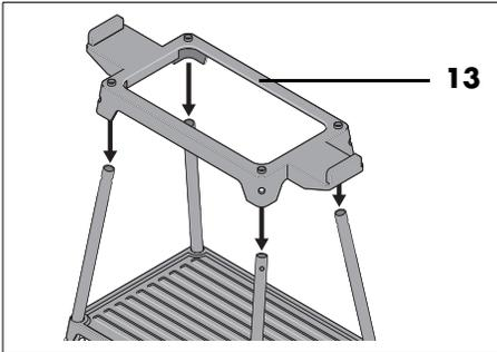
4. Put on the frame **13** and fix it with screws **22** and wing nuts **21**.
