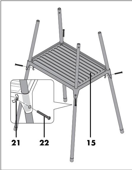
3. Push the legs through the shelf **15**. Insert one screw **22** each and fasten with the wing nuts **21**.
