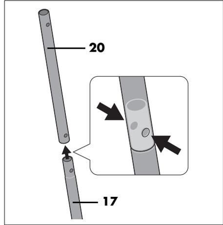
1. Long rod **17** into short rod **20**. The holes are exactly on top of each other.
