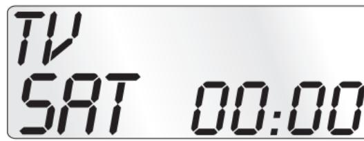
The standard readout of the LCD display ① consists of the details for the relevant device, for example, "TV", the initial for the day of the week and the time of day indicator.
