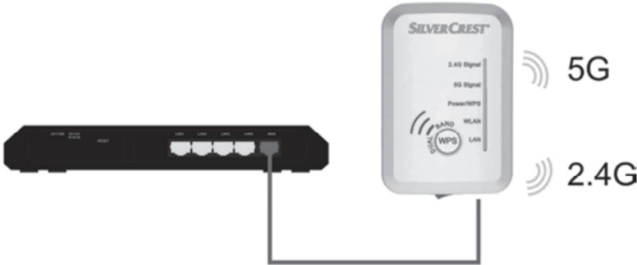
The mode selector (10) must be set to the "Access Point" position for AP Mode.
