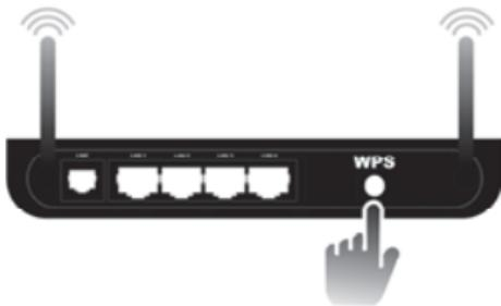
(Symbolic representation, connection button (WPS) can be differently arranged and referred to depending on the router model.)
