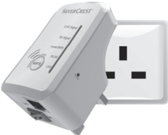
Then switch on the dual-band wifi range extender by turning the main switch (9) to the "ON" position. The dual-band wifi range extender requires a certain amount of time (boot time) after it is switched on before it is ready to use. The Power/WPS LED (3) lights up permanently as soon as the booting process is complete.
