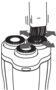
Remove the protective cover [1]. Then clean the shaving heads of the shaving system [2] with the enclosed cleaning brush.
