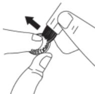
Remove the razor blade from the guard. Then clean the razor blade carefully with the enclosed cleaning brush.
