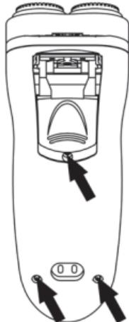
Pull out the trimmer [6]. Remove the three screws and open the casing.
